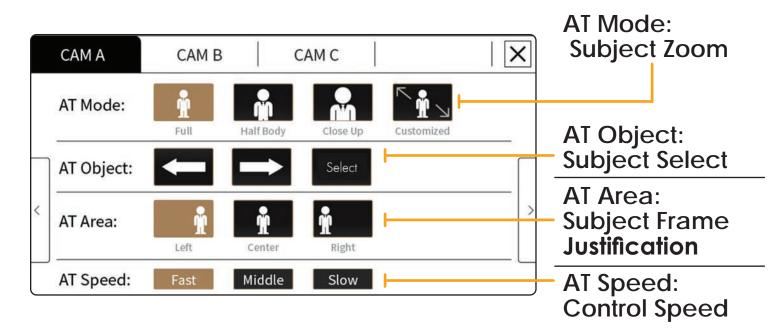
Datavideo's unique tracking camera control can be achieved through production switchers, presentation switchers, PTZ camera controllers and apps eliminating IR remote or WebGUI controls.
